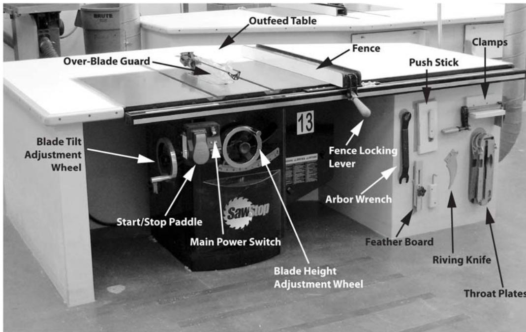
Although the table saw is one of the most useful machines in the Makerspace, it is also one of the most dangerous. It can be used to accurately rip and crosscut lumber and sheet goods. The table saw can also be used for special operations including cutting dadoes and rabbets and for resawing. With the use of special jigs, joinery like tenons and box joints can be made. In addition, the blade can be tilted for cutting bevels and miters.
